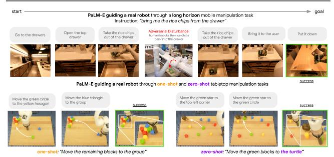
Figure 5: A single PaLM-E model directs the low-level policies of two real robots. Shown is a long-horizon mobile manipulation task in a kitchen, and one-shot / zero-shot generalization with a tabletop manipulation robot.
